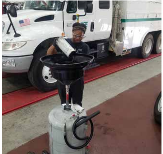
Intern Justice Mckeever drains excess oil from an oil filter after conducting a routine preventive maintenance oil change on an overhead operations truck at the RBC maintenance facility.
